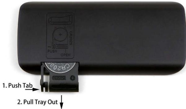
To replace the remote battery, place the remote face down, push the small tab to the right and then pull the battery tray out. Place one CR2025 lithium button-cell battery on the tray with the positive “+” side facing you. Reinsert the tray.
