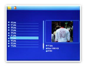
delete files and folders from a storage drive instead since a computer is much faster and more convenient. To delete a file or folder, highlight it using the cursor and press the "Right" button to bring up the deletion menu. Press the "Play/Pause/Enter" button once to initiate deletion, and once again to confirm.
