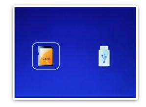
To select a storage device, press the "Menu/Return" button repeatedly until the storage selection screen is shown. Highlight the desired storage device and press "Play/Pause/Enter" to select it.
