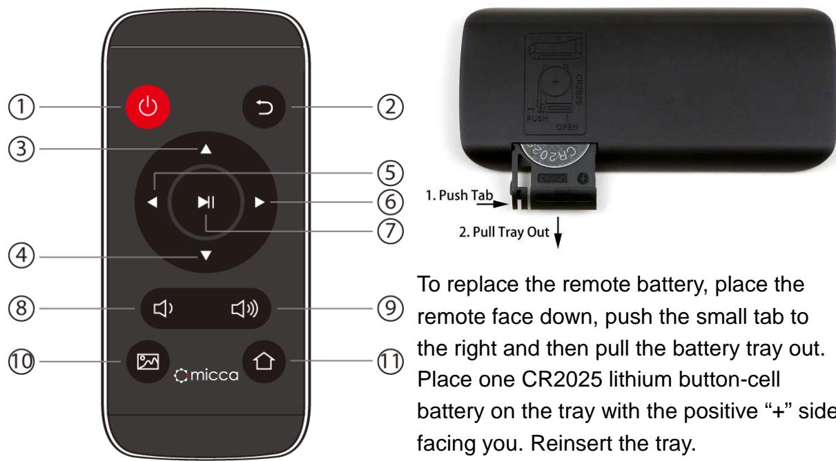
To replace the remote battery, place the remote face down, push the small tab to the right and then pull the battery tray out. Place one CR2025 lithium button-cell battery on the tray with the positive "+" side facing you. Reinsert the tray.
